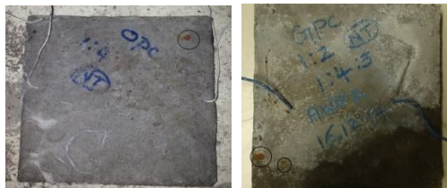
Figure 8. Corrosion spots formed in specimens
