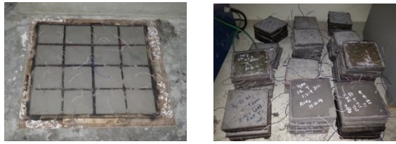
Figure 7. Ferrocement panels left for drying
