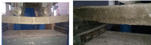
Figure 3. Initial crack and Failure of panels
