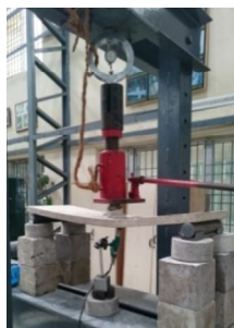
Figure 4. Test setup of Ferrocement slabs
